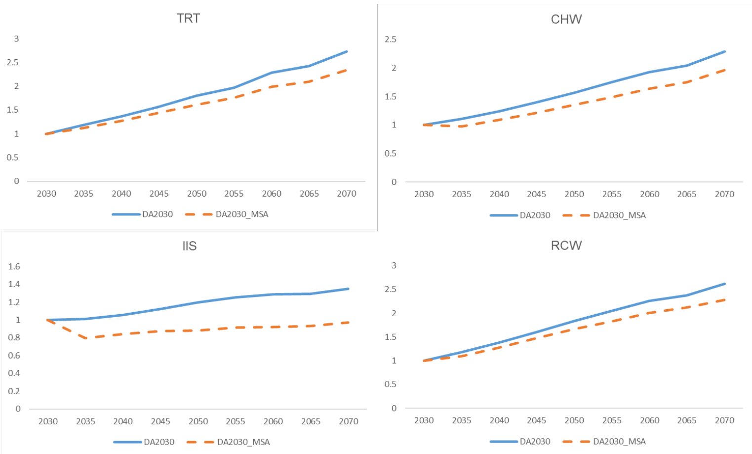
Figure A2: Comparison of demands (a) Car road (b) Commercial hot water (c) Iron and steel (d) Residential clothes washing, for the DA2030 scenario in linear and MSA versions of TIAM-UCL (indexed to 2030)
