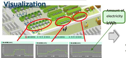
Visualize the electricity use of each production process and production
