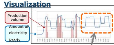
Visualize the electricity amount and production volume shows us the useless point of electricity use.
