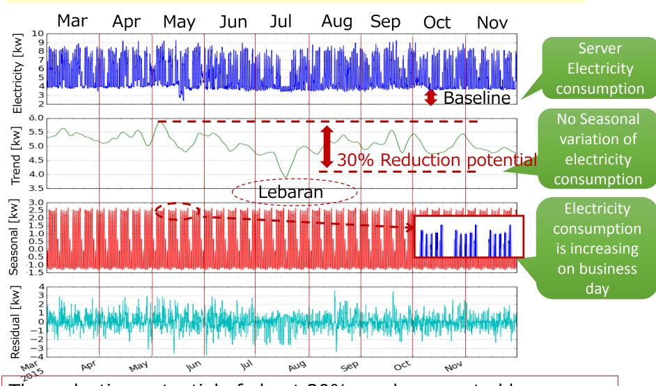
The reduction potential of about 30% can be expected by improving equipment and thermal insulation performance
