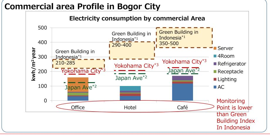
Monitored Commercial Area consumes Electricity lower than Green Building Index in Indonesia (*Better* than Green Building). The usage rate of the air conditioner is high (End Use).
